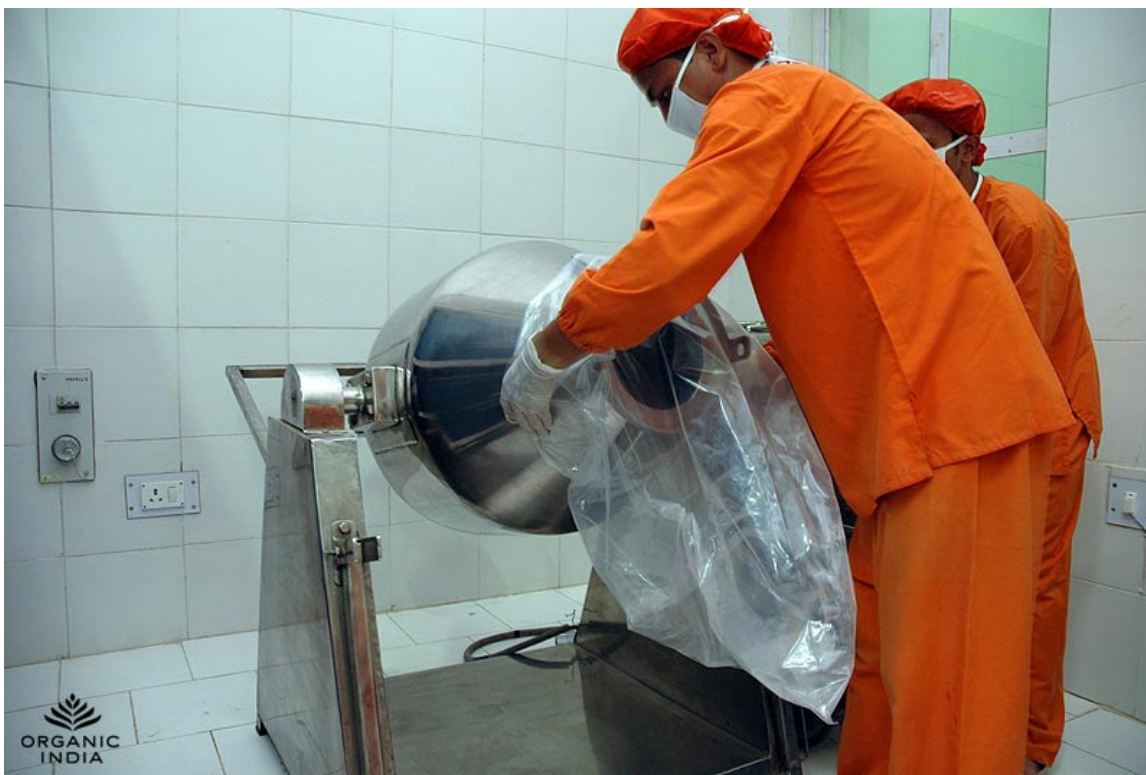
OFF-LOADING OF TULSI LEAVES FROM THE CONE BLENDER Organic India® Lucknow Production Unit January 2007
