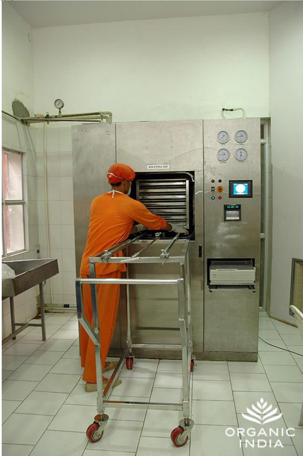
LOADING OF TULSI LEAVES INTO THE STEAM DISINFECTION MACHINE Organic India® Lucknow Production Unit January 2007
