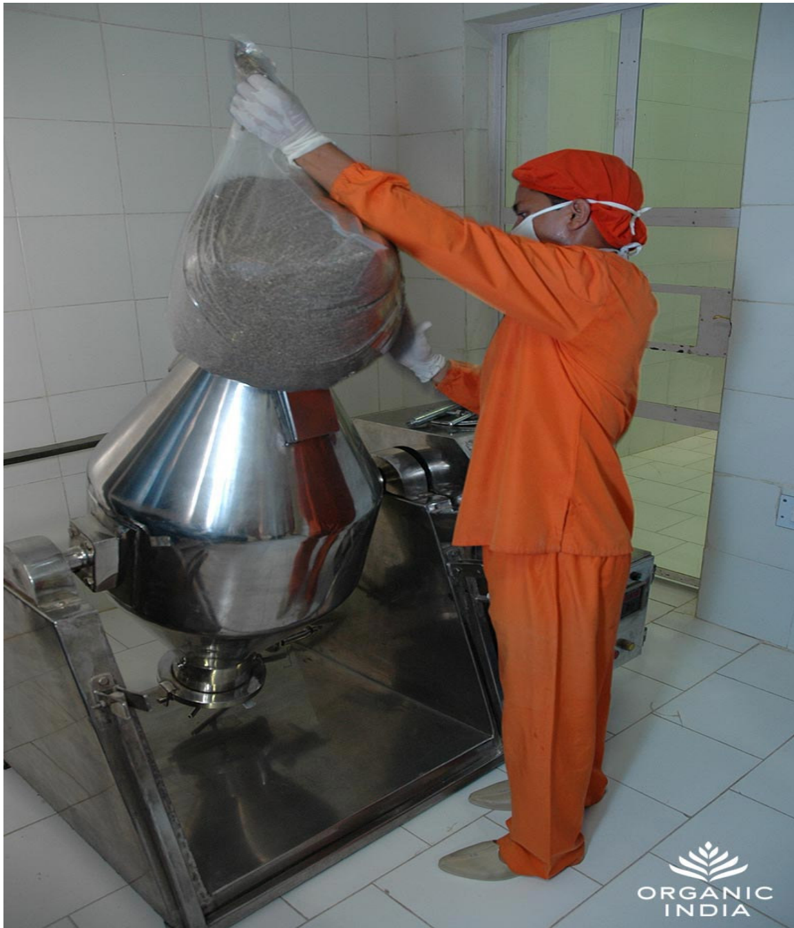
FEEDING THE TULSI INTO THE CONE BLENDER Organic India® Lucknow Production Unit January 2007
