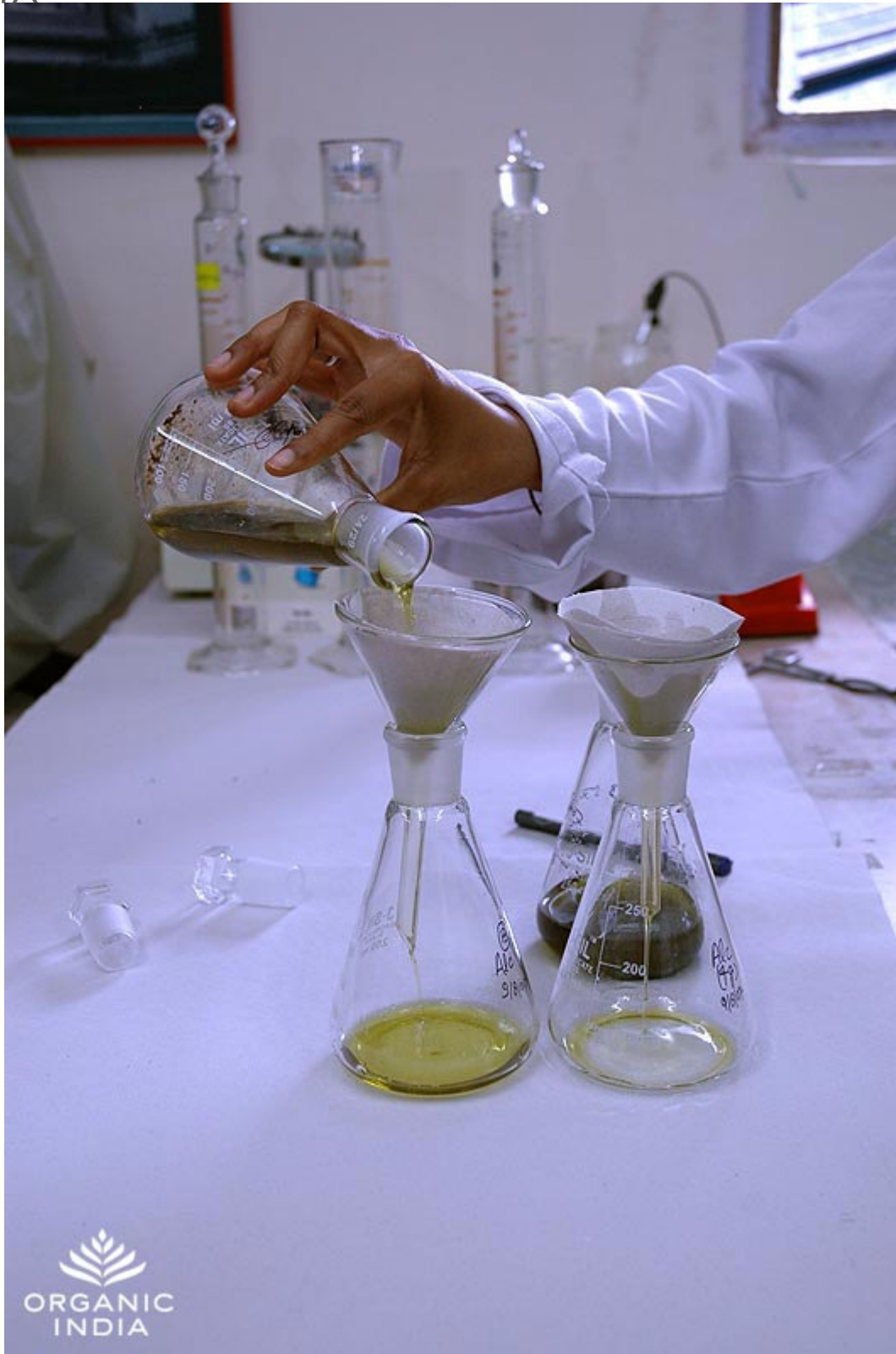
DETERMINATION OF ALCOHOL EXTRACTIVES IN TULSI IN PLACE Organic India® Lucknow Production Unit January 2007
