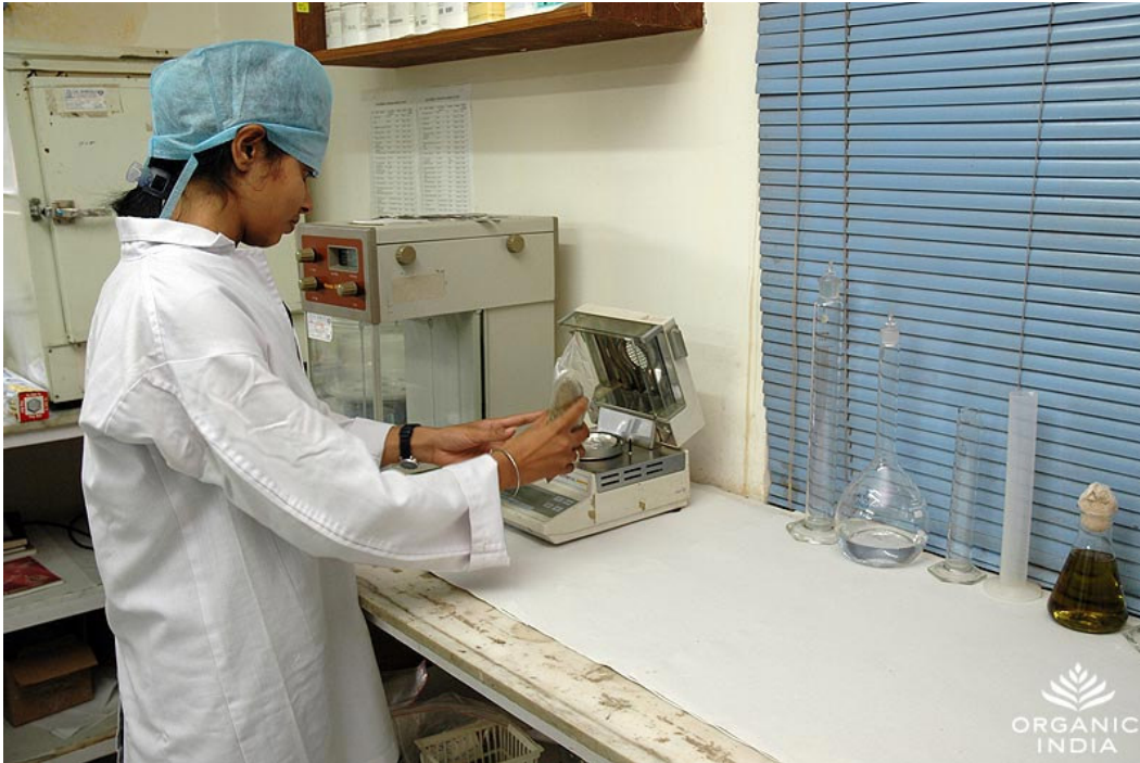
DETERMINATION OF MOISTURE CONTENT Organic India® Lucknow Production Unit January 2007
